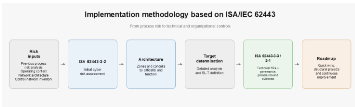
Figure 2: Recommended sequence for implementing Zero Trust and Defence in Depth controls through ISA/IEC 62443.
