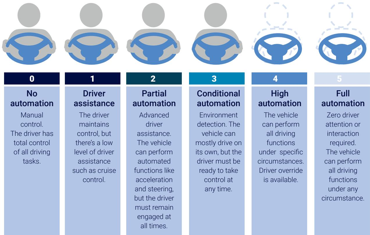
Figure 1: The levels of driving automation<sup>1</sup>
