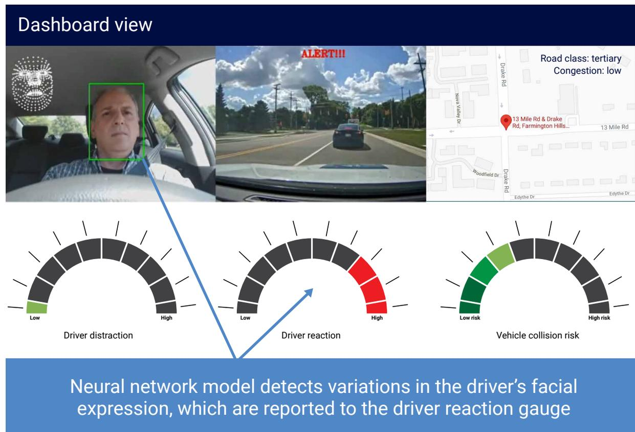
Figure 5: Dashboard view of a driver's response to a critical driving event
